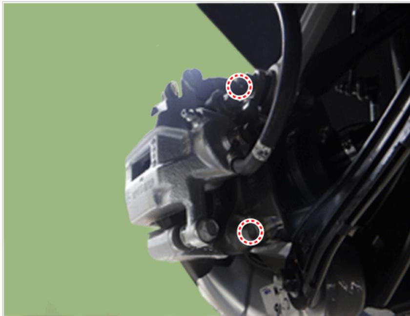
3. Loosen the brake disc screw and then remove the brake disc.
